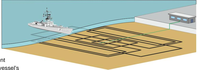
The greater the depth of water the greater the current required to achieve the magnetic field levels at the vessel's hull necessary to modify the magnetisation and provide the required level of signature reduction.
