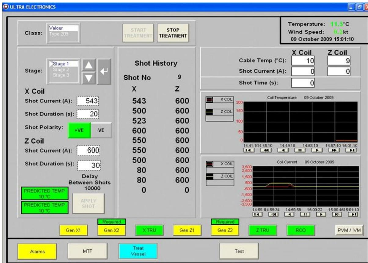
Main Control Panel showing the Treatment Pulse Sequence
