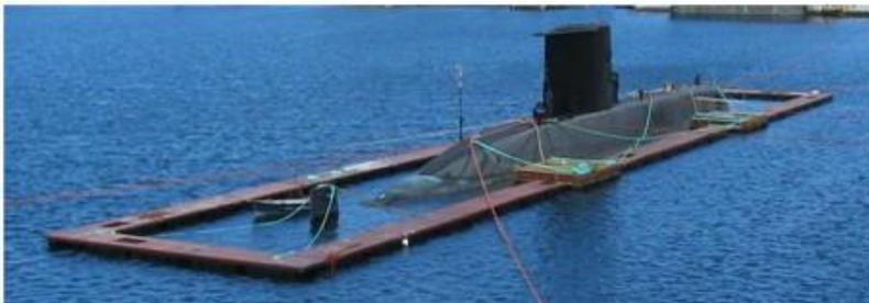
Close-Wrap systems have configurable coils sets to treat both ships and submarines and can be supplied in various formats from fixed, permanent systems to fully portable systems with floating coils with independent power supplies. The treatment has a long lasting effect for all vessel types.
