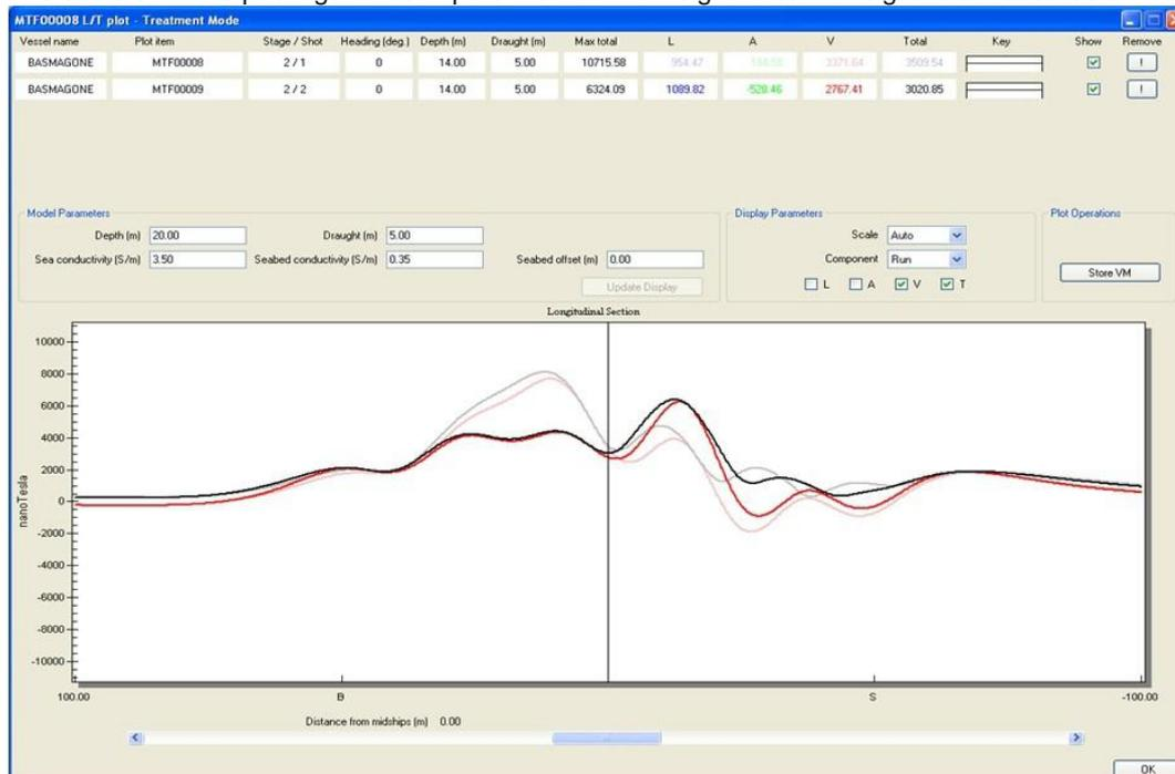
Comparison of the signatures measured with the previous pulses (Drive-In or Close-Wrap) or transits (Over-Run)
