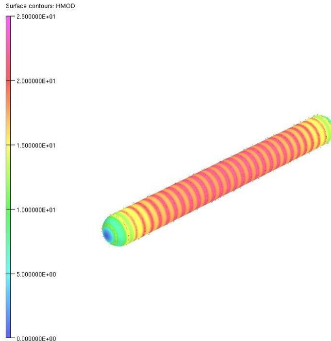
*Uniform magnetic field of an X coil (in red) designed for a close wrap treatment of a submarine*
