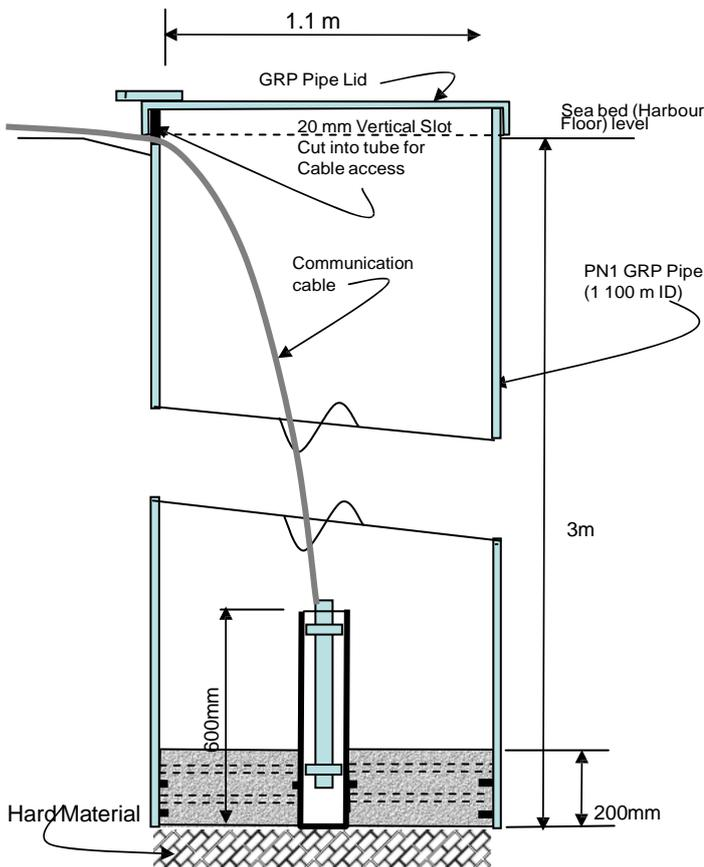
Diagram shows a cross section through the sensor mount.
