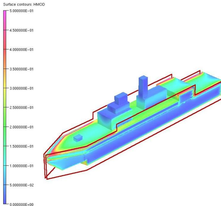
*Uniform magnetic field of a Special Y coil pair (in red) designed for close wrap treatment of a surface ship treated on a non-ideal heading*
