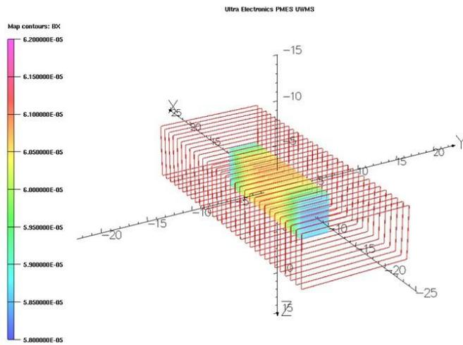
'L' coil (in red) showing the field uniformity at the ship's location
