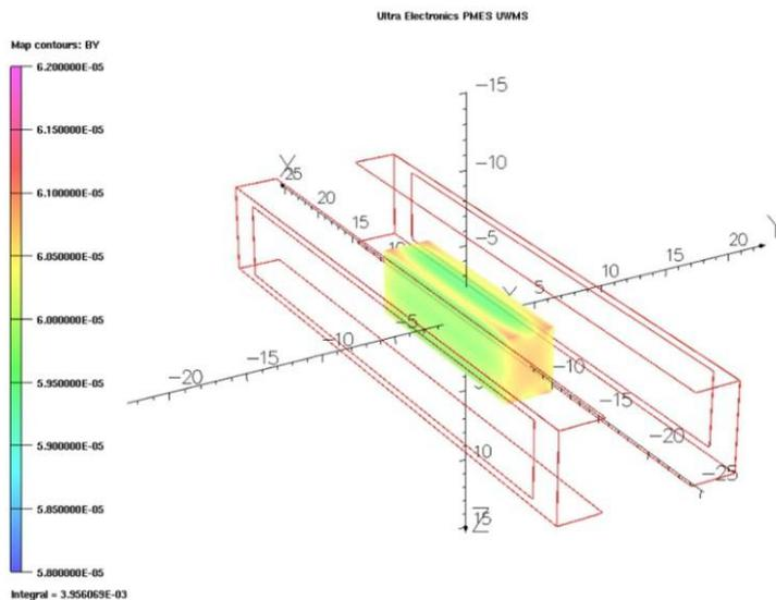
A complex 'Y' coil (in red) designed for high magnetic field uniformity at the ship's location
