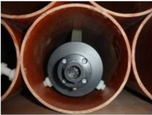
Diagram shows a 3-axis magnetic sensor viewed from inside the sensor mounting tube. The sensor mounting tubes are sunk into the sea bed and the magnetic sensor positioned in the tube.
