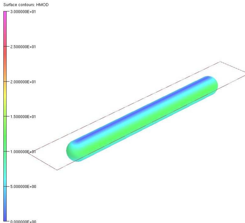
*Uniform magnetic field of an Floating Z coil (in red) designed for a close wrap treatment of a submarine*
